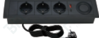
BFF-1112 Material: Aluminum Alloy, ABS Configurations: 3×German Socket 1×USB Type-A 1×USB Type-C 1×Wireless Charger Panel Size: 298*70mm Hole Size: 280*65mm
