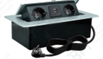
BFF-1222 Material: Aluminum Alloy, ABS Configurations: 2×German Socket 2×USB Type A Panel Size: 265*118mm Hole Size: 225*115mm
