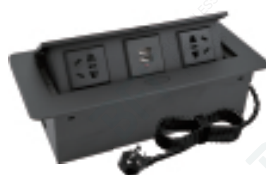
BFF-1214 Material: Zinc Alloy, Iron Configurations: 2×CN Five-plug Power Socket 2×USB Type A Panel Size: 265*118mm Hole Size: 225*115mm
