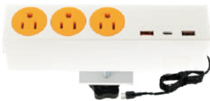
BFF-1812 Material: ABS Configurations: 3×American Socket 2×USB Type-A 1×USB Type-C Panel Size: 200*42mm
