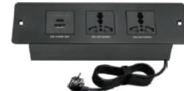
BFF-1110 Material: Aluminum Alloy Cold Rolled Steel Configurations: 2×Universal Socket 1×USB Type-A 1×USB Type-C Panel Size: 220*63mm Hole Size: 185*55mm
