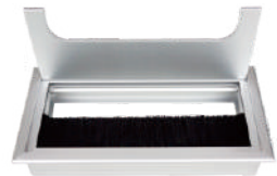
BFF-1930 Material: Aluminum Alloy Panel Size: 160*80mm Hole Size: 150*70mm Color: Silver/Black Finish
