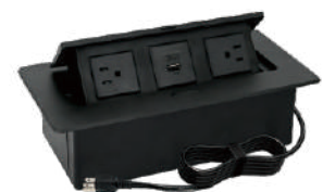
BFF-1204 Material: Aluminum Alloy, ABS Configurations: 2×American Socket 1×USB Type-A 1×USB Type-C Panel Size: 265*133mm Hole Size: 225*115mm
