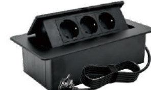
BFF-1240 Material: Aluminum Alloy, ABS Configurations: 3×German Socket Panel Size: 265*133mm Hole Size: 225*115mm
