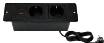
BFF-1107 Material: ABS Configurations: 2×German Socket 1×USB Type-A 1×USB Type-C Panel Size: 195*60mm Hole Size: 155*55mm
