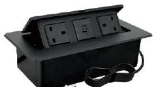
BFF-1205 Material: Aluminum Alloy, ABS Configurations: 2×UK Power 1×USB Type-A 1×USB Type-C Panel Size: 265*133mm Hole Size: 225*115mm
