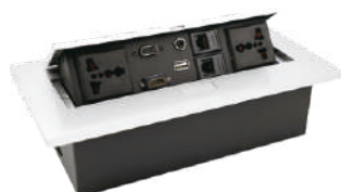
BFF-1216 Material: Zinc Alloy, Iron Configurations: 2×Universal Power, 1×Network 1×Telephone, 1×VGA, 1×3.5Audio 1×HDMI, 1×USB Data Panel Size: 265*118mm Hole Size: 225*115mm
