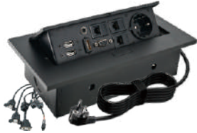
BFF-1218 Material: Zinc Alloy, Iron Configurations: 2×German Socket 2×Network, 1×Telephone 1×VGA, 1×HDMI 2×USB Data, 1×3.5Audio Panel Size: 265*118mm Hole Size: 225*115mm
