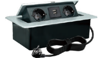
BFF-1221 Material: Aluminum Alloy, ABS Configurations: 2×German Socket 2×USB Type A Panel Size: 265*133mm Hole Size: 225*115mm
