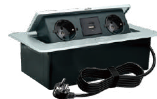
BFF-1221 Material: Aluminum Alloy, ABS Configurations: 2×German Socket 1×USB Type-A 1×USB Type-C Panel Size: 265*133mm Hole Size: 225*115mm
